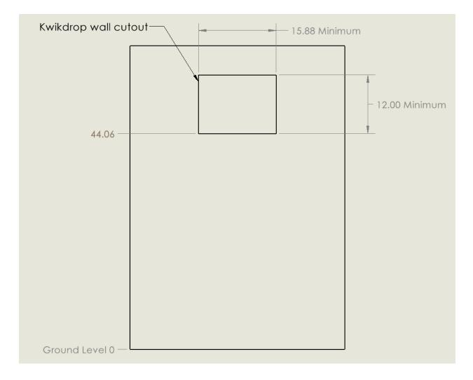
The above instructions are based on the interior and exterior grades being at the same level. Please note that the measurement from the ground level to the bottom of the depository opening must be 48" so that the thru-wall unit will be ADA compliant and to allow sufficient clearance for the Kingsley ballot carts.
