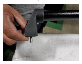
3. Insert Bolts of the handle assembly through the holes on the same side of cart that the swivel casters are on. Attach hardware using a  $\frac{1}{2}$ " socket or wrench and tighten as shown below.
