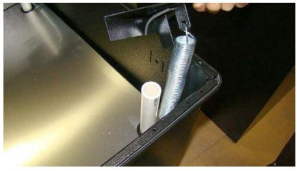
**STEP 3:** Remove the springs from each of the four corner gussets with pliers as shown below.
