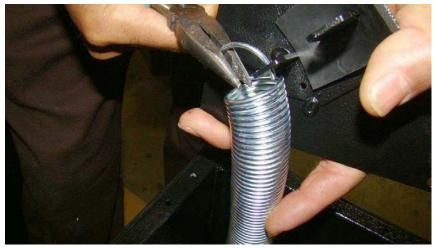
**STEP 4:** Remove the springs from each of the four corner eye bolts located on each corner of the float tray with pliers as shown below.
