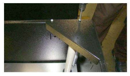
**STEP 2:** Remove each of the four gussets in an upward motion disengaging the white float tray guide from the gusset as shown below.
